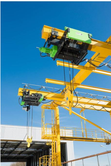
You won't find these wire rope hoists in any catalogue: STAHL CraneSystems developed the customised hoists to meet the requirements of CraneBuilders and Deltares.
