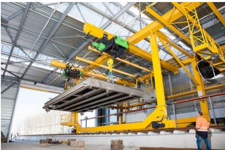
The wire rope hoists can be coupled for tandem operation, for example to lift the partition wall for shortening the flume. Lateral jibs enable loads to be taken up outside the gantry crane.
