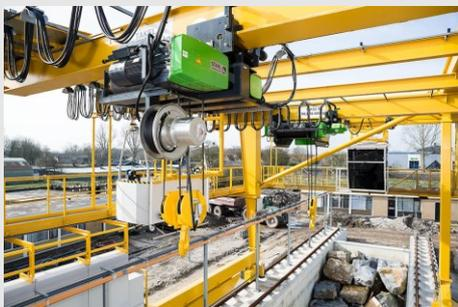
This wire rope hoist has been developed to assist the scientists building the test dykes with its fast, precise lifting movements.
