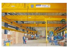
Lifting at three levels: here semi-portal cranes, bridge cranes and bracket cranes work in parallel.
