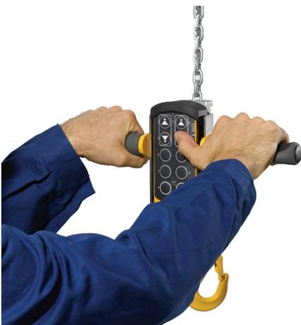
Guiding the load safely with both hands. Operating the hoist is possible for both right- and left-handed users.
